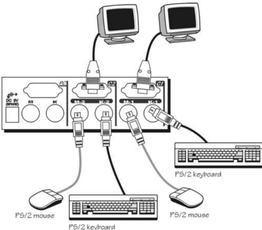
Figure 1: Console Connection
